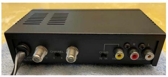
This Radio Shack RF modulator can provide an NTSC type RF signal to older TVs or video monitors that require an analog signal as an input. The output is user-selectable for either channel 3 or channel 4 output and can provide 75 ohm or 1k ohm impedance. Input is AV video/video using standard phono-type plug cables. An RF coax jumper cable is provided.
