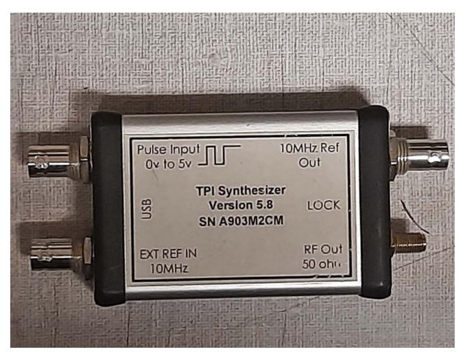
It is the same Analog Devices frequency chip inside, but also has a USB interface and 10 MHz output. A bit of Google-foo, and I found the original manufacturer. Went to **rf-consultant.com** and downloaded the control software. Did not work, so I sent the website contact an email. The next day, the **owner** sent me the correct program for a 10+ year old product, including the calibration for this serial number. **Works**!
