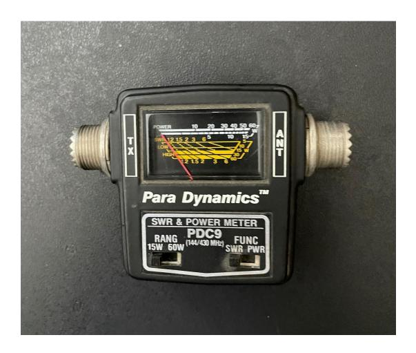
The Para Dynamics PDC9 inline SWR / Power Meter operates from 144MHz to 430MHz which includes the 2m - 70cm ham bands. The unit has two power ranges, 15W and 60W. Unit provides two female SO-239 coax connectors. Unit measures approximately 2" X 2.5" X 1". A similar unit recently sold on eHam.net for \$25.
