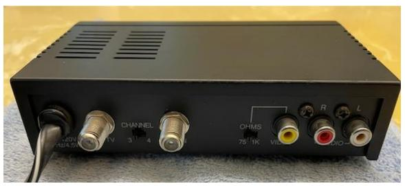
This Radio Shack RF modulator can provide an NTSC type RF signal to older TVs or video monitors that require an analog signal as an input. The output is user-selectable for either channel 3 or channel 4 output and can provide 75 ohm or 1k ohm impedance. Input is AV video/video using standard phono-type plug cables. An RF coax jumper cable is provided.
