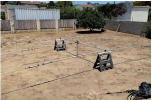
Then I tested the final assembly with my NanoVNA. I knew from my research that testing at ground level wouldn't be the same as testing at height, but it would let me know if anything was hideously wrong.
