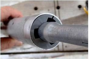
While I was 3D printing things, I designed and printed a little tool that allowed me to mark the assembly points on the traps.
