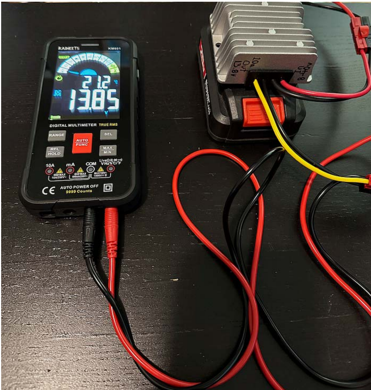
Multimeter showing output voltage of The Bauer-Pack with the 13.8v buck converter
