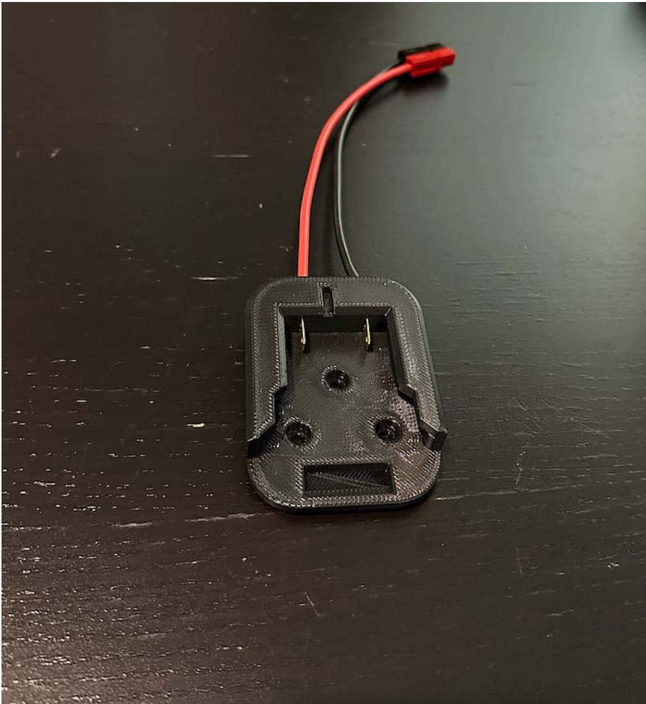
Battery output adapter with attached Powerpoles
