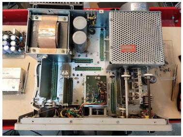
All the cards. Get out the eraser scrubber! All dirt, corrosion, and oxidation must be banished.
