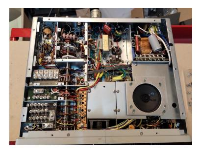
All the cards removed. Gold fingers on the edge connectors, but tin plating on the cards.
