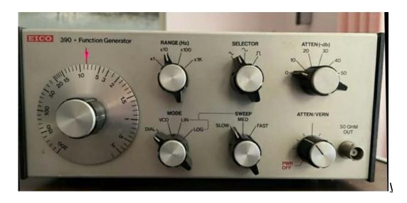
This function generator can provide sine wave, triangular wave or square wave outputs with a frequency range of 0.2 Hz to 200 KHz selectable over 4 ranges. Output waveforms can be selected to perform a wide variety for testing of electronic equipment. Output up to 10 v p-p is provided which may be attenuated from 0 to -50 dB. This unit also provides a sweep generator which can provide linear or logarithmic sweep modes of up to 1000:1 sweep range with a choice of three different sweep speeds.
