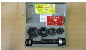
Deep throat hole punch (like Whitney), for thin sheet metal.
