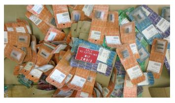
Heat shrink tubing. Heat shrink tubing, lots of colors. Ask for a baggie of assorted bits. I for instance, put Yellow for "Yeasu" on my long whip antenna.
