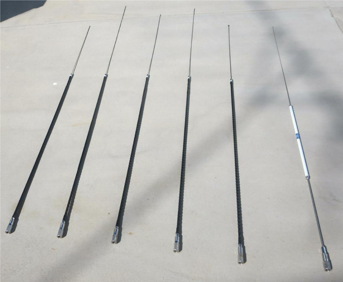
I have five MFJ 1/4 wave hamstick-type antennas for sale, ranging from 75m, 40m, 20m, 15m and 10m plus a 5/8 wave Hustler CG-144 for operation on 2m. All of them feature a standard 3/8-24 threaded mount with a Hustler QD-2 quick disconnect adapter installed for quick R&R when operating on different bands. Typically the MFJ hamsticks sell for around \$30 new, the Hustler 2m antenna currently lists for \$73 while the Hustler QD-2 quick disconnect adapters sell for \$35 per set.
