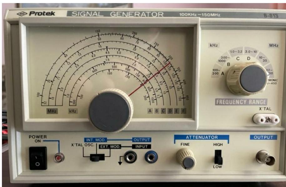
This signal generator provides an RF sine wave signal from 100 kHz to 150 MHz over 6 different frequency ranges. The output level can be adjusted from 30 mV to 250 mV RMS Max via the attenuator control. The unit also allows a 1 MHz to 15 MHz external crystal to be used for operation on a fixed frequency in lieu of VFO operation. Output is modulated at a 1 kHz signal at a 1V RMS level.
