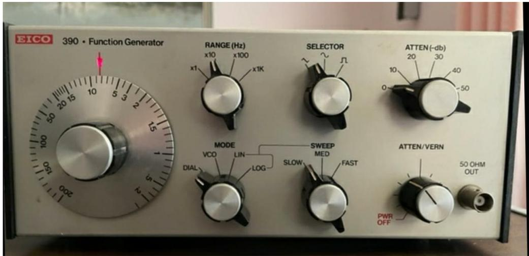
This function generator can provide sine wave, triangular wave or square wave outputs with a frequency range of 0.2 Hz to 200 KHz selectable over 4 ranges. Output waveforms can be selected to perform a wide variety for testing of electronic equipment. Output up to 10 v p-p is provided which may be attenuated from 0 to -50 dB. This unit also provides a sweep generator which can provide linear or logarithmic sweep modes of up to 1000:1 sweep range with a choice of three different sweep speeds.
