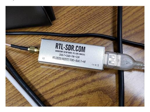
This particular one is considered higher quality than most, and as a result is a bit more expensive: \$25:-) Most of them have a connector for an external antenna but this particular one has an SMA connector. It also has a metal enclosure, which provides better shielding than a plastic enclosure, which many of them use.
