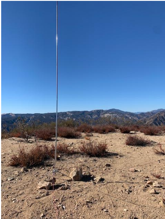
Vertical Telescoping Antenna with wire radial ground plane
