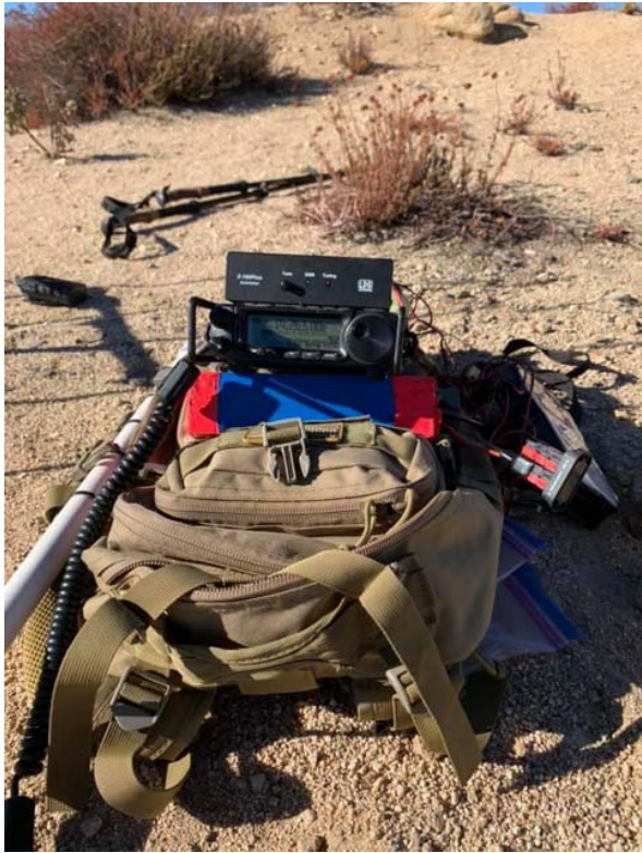
Vertical Telescoping Antenna with wire radial ground plane
