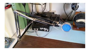
Here is the electret microphone element. Same thing as in almost every hand microphone, so no changes to the radio. The blue foam disk is a 3M scrubbie pad, and some white packing foam inside to dampen out echos. Peeking out from behind the foam is a tiny orange capacitor required by the microphone.
