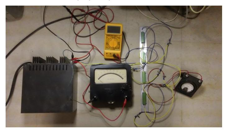
Of course I had a digital volt meter on the test, but the analog meters shown below were of more interest. As I switched the load between values, I watched the voltage to make sure it kept steady regulation. The digital voltmeter has a slower update rate that might not show a voltage fluctuation.
